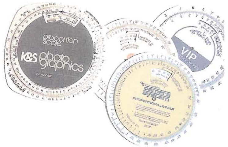
Figure 5-43. A sampling of proportional scales used to determine reproduction sizes for photographs or for other illustrations.
