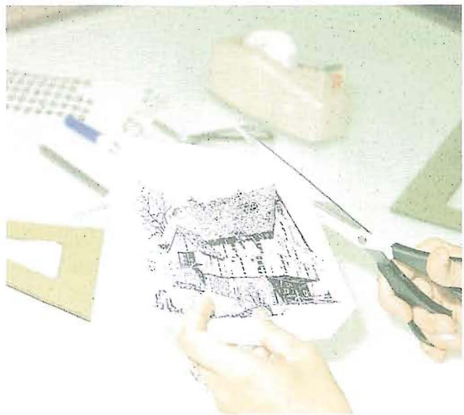
Figure 5-46. Line art is drawn to the necessary size and pasted up on the mechanical.
